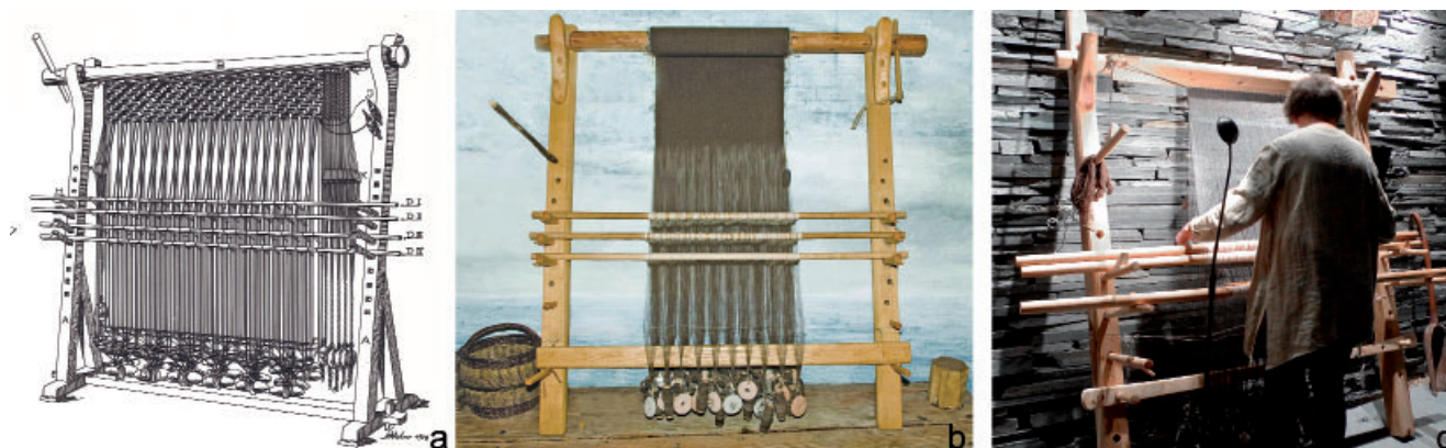
Fig. 3: Methods for weaving 2/2 twill using one or two warps per heddle and a varying number of single-notched support pairs: a) proposed method for weaving the Thorsberg mantle: one warp per heddle, four support pairs, four heddle rods (after Schlabow 1952); b) weaving sailcloth at the Viking Ship Museum: two warps per heddle, three support pairs, three heddle rods (Image: Werner Karrasch, © Viking Ship Museum, Roskilde); and c) weaving diamond twill at the Lendbreen tunic exhibit, Norsk Fjellmuseum: two warps per heddle, two support pairs, three heddle rods (Image: Randi Andersen, Osterøy Museum)
