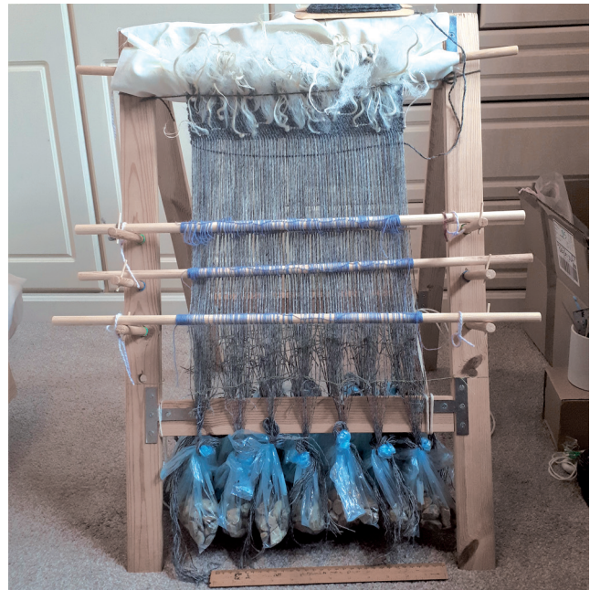
Fig. 3: The small-scale warp-weighted loom used to weave the textile samples (Image: Julia Hopkin)
