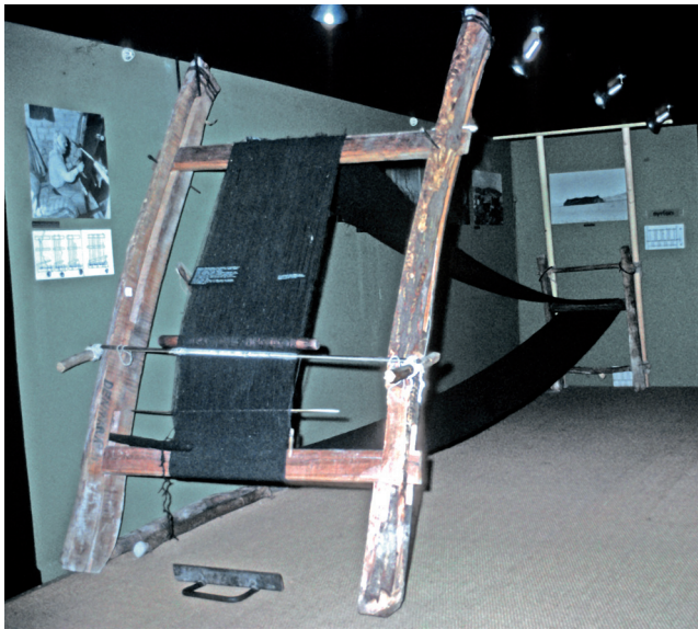
Fig. 8: Three beam-loom set up with a tubular goat hair warp for tent canvas. The loom was acquired by Hald in Syria in 1960 and belongs to the National Museum, Copenhagen, where it was exhibited in 1967. (Slide no. 550 in CTR's collection)
