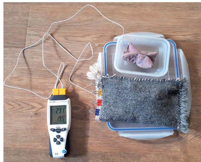
Fig. 6: The equipment used for testing the samples' insulation properties, showing sample 1 with a heat pack inside, the uninsulated heat pack used as a control, and the dual probe thermometer used to measure the temperature of both heat packs from outside the refrigerator (Image: Julia Hopkin)
