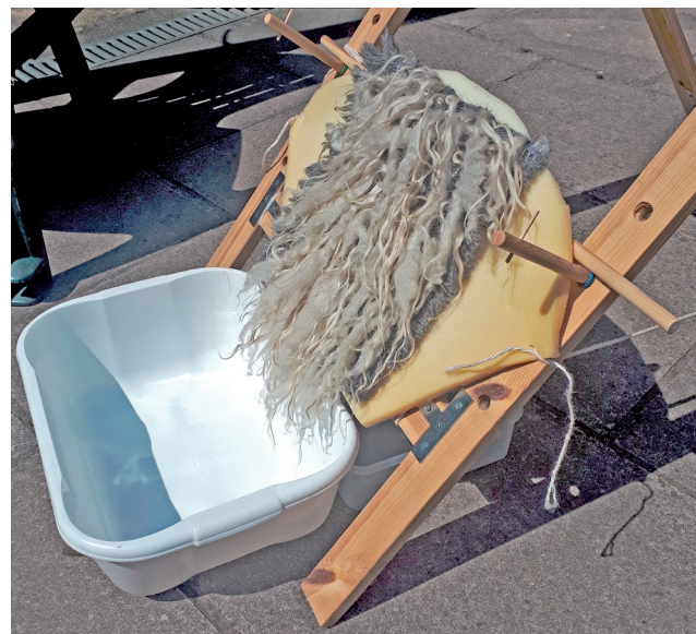
Fig. 7: The equipment used for the water resistance experiment showing sample 3 attached to a layer of foam, mounted at approximately 45° on a wooden frame, with a bucket placed underneath to collect water which ran off the sample (Image: Julia Hopkin)
