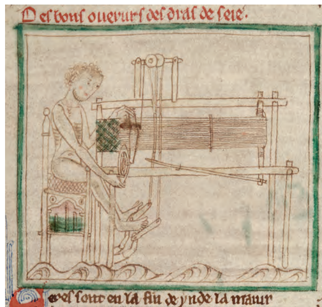
Fig. 2: A 13th century depiction of the horizontal treadle loom in use. Cropped detail from the Romance of Alexander O.9.34, f032v (Image: © The Master and Fellows of Trinity College Cambridge, reproduced with permission)
