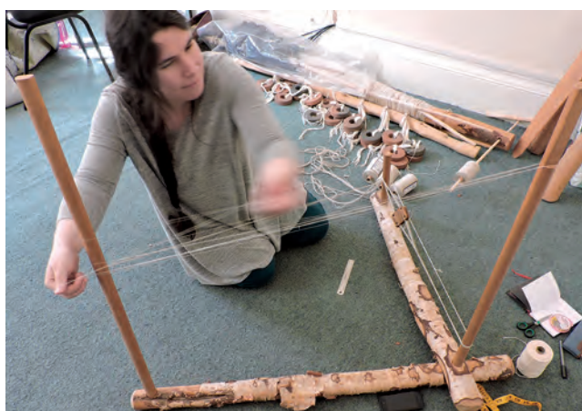
Fig. 6: Warp for the warp-weighted loom being wound on a warping frame (Image: Ellie March)
