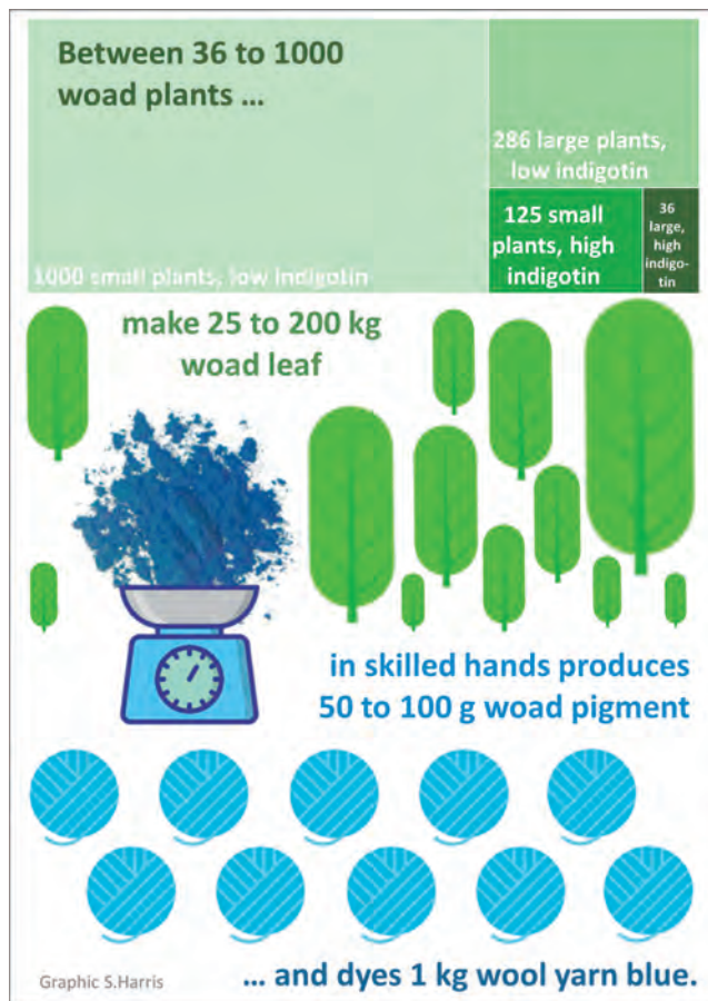
Fig. 9: Summary of results: how many woad plants does it take to dye 1 kg wool yarn blue? (Image: © Susanna Harris)
