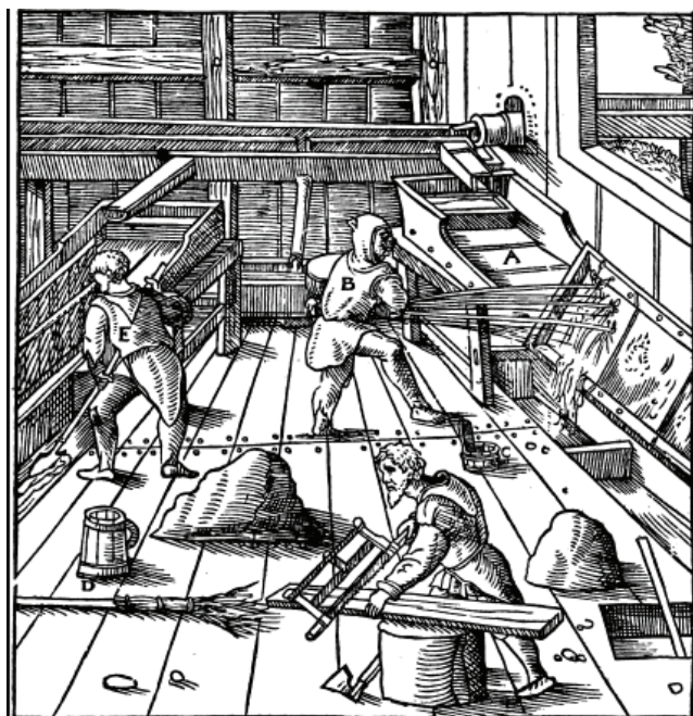
Fig. 18. Etching from De re metallica , illustrating the sluice. A: Table, B: Wet textiles, C: Bucket, D: Other type of bucket, E: Remains of veined ore rock (After: Agricola 1530, 243).
