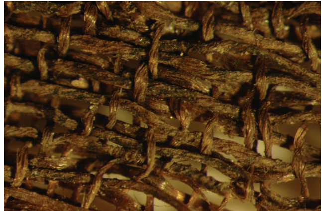
Fig. 11. In this detail traces of the membrane gold is visible in some places as a semi-transparent dark coating of the silk yarn. An s-twist of the silk core is discernible (Photo: Irene Skals).
