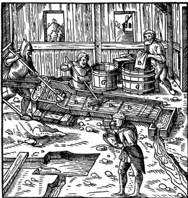
Fig. 16. Etching from De re metallica , illustrating the sluice. A: Table, B: Textile, C: Top of the table, D: Pipes, E: Settling tank, F: Rake, G: Tank (After: Agricola 1530, 242).
