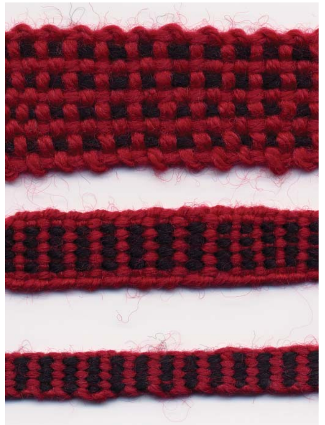
Fig. 6. Three bands made using the same heddle and tapestry wool yarn. Plain weave, warp dominant weave and warp faced (© Susan J. Foulkes).
