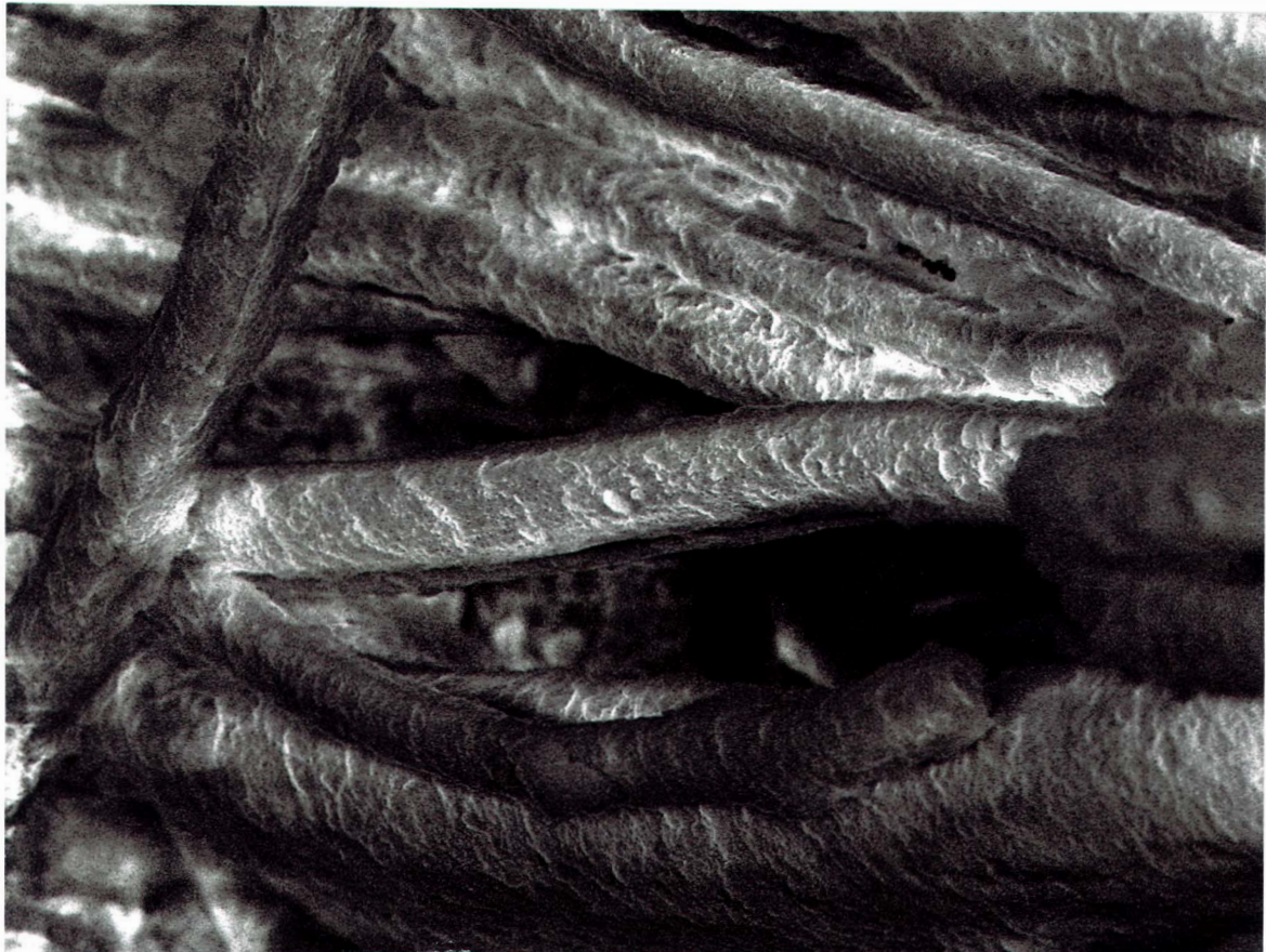
Fig.2 Typical wool scales seen after rinsing in de-ionized water in an ultrasonic bath for four minutes. (SEM photo: Anita Malmius and Malgorzata Wojnar-Johansson)
