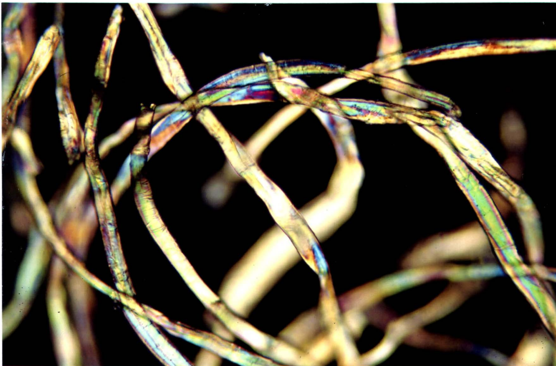
Fig.21 Separated cotton fibres from D13 B (above), as seen in the polarising microscope 220x (Photo: R. Oldfield)
