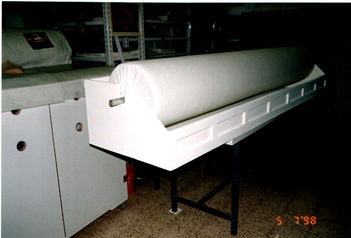
Fig.4 'Wrapping sheet' rolled in plexiglass cylinder set in special container.
