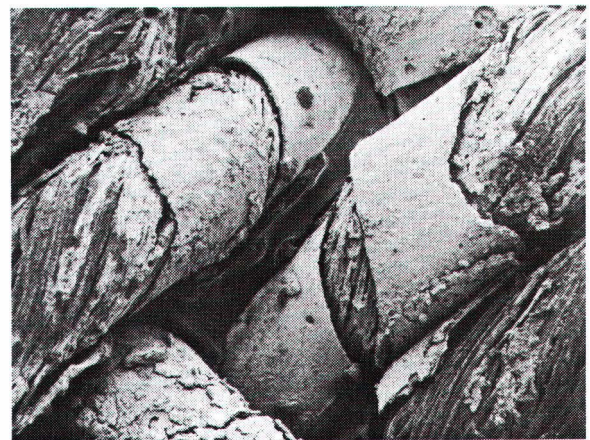
Figure 2 Detail of the degraded metal warp on the yarns within the bracelet. Some portions of the metal are quite well preserved and show the straight, cut edge of the metal ribbon. (64x, SEM photomicrograph: Trevor Jones, UMIST.)
